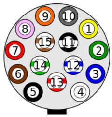
Figure 4: LV Connector acc. ISO 12098
