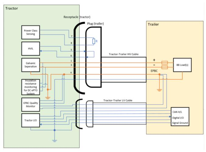
Figure 2 HV and LV connectors
