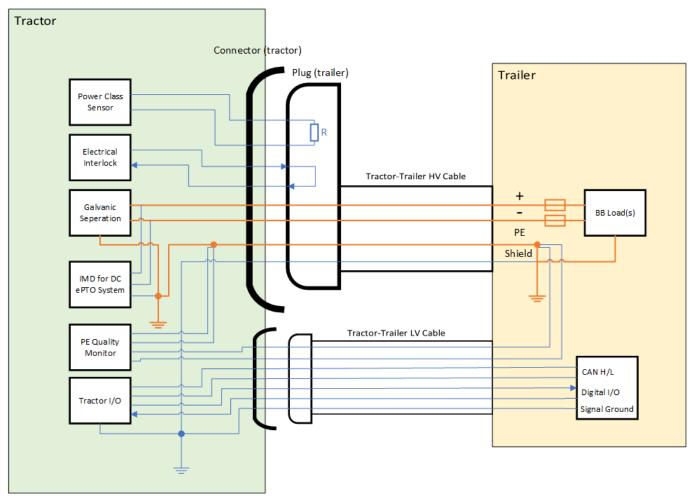
Figure 4 HV and LV connectors
