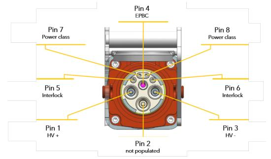
Figure 5 HV Connector acc. AEF
