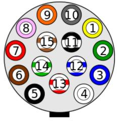
Figure 6: LV Connector acc. ISO 12098
