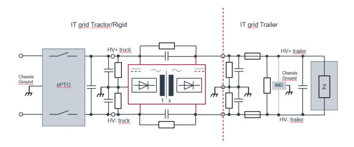
Figure 1 Wiring diagram for HV galvanic separation of truck and trailer
